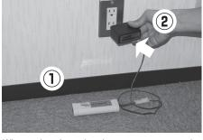
When charging the battery, connect the battery to quick charger, then plug the charger into an outlet. It will take about 70 minutes to fully charge the supplied battery.
