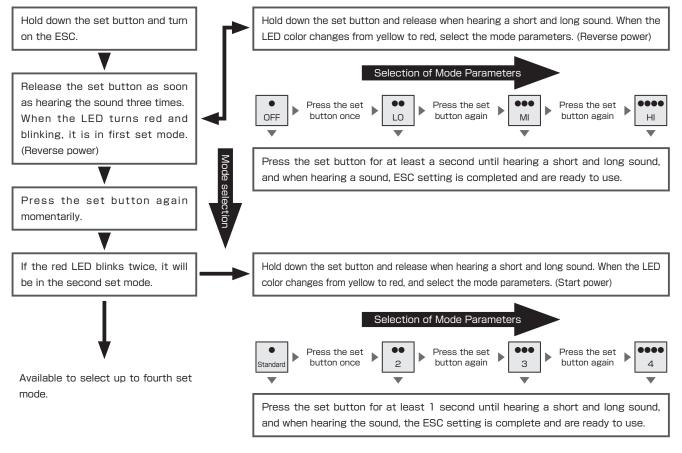
The above instructed LEDs are built into ESC. The other LEDs installed in ESC only lights up in red.
