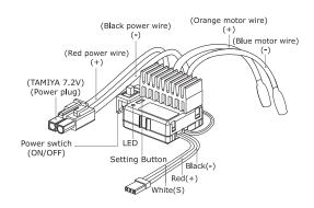
The receiver connector connects to CH2. The polarity matches Sanwa, KO and Futaba receivers. Check the polarity for other brands of receivers before plugging in.
